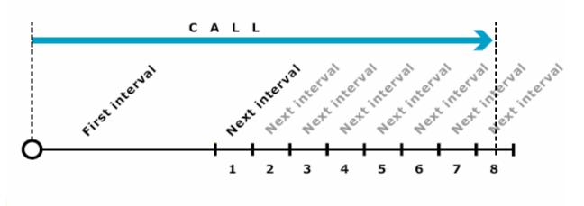
The figure above demonstrates how calls are charged. All calls shorter than the *First interval* will be rounded to First interval seconds. Calls longer than *First interval* will be rounded up to multiple Next interval seconds. The call illustrated in the figure above will be charged using the following formula:
